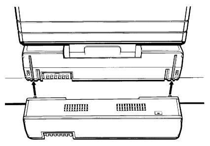
5. Pull the battery pack up until it snaps into place.
